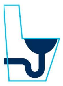
A P-trap is another common type of toilets. It gets its name from the fact that it uses a "P" shaped pipe to connect to the sewer line.
