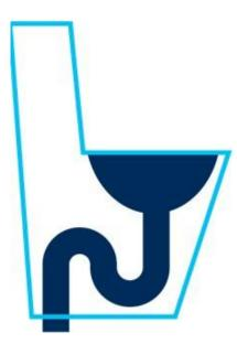
The s-trap is the most common type of toilets. It gets its name from the fact that it uses a "S" shaped pipe to connect to the sewer line.
